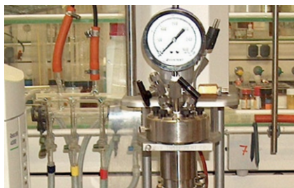
In situ high pressure infrared spectroscopy to monitor catalytic conversions
