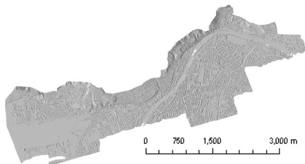
Fig. 1. Shaded relief map of the last echo DSM of the autumn flight showing the test site of Innsbruck (Austria) where multi-temporal airborne laser scanning data is available
