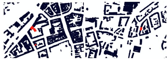
Fig. 7. Automatically detected locations of changed buildings with two zoomed-in examples from the city centre
