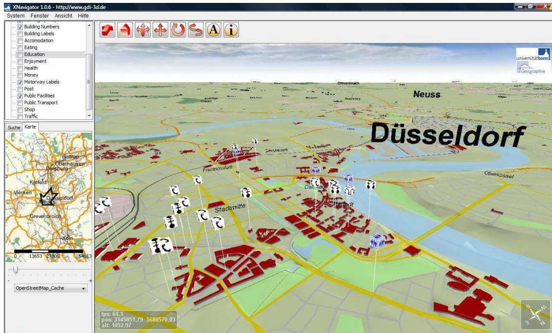
Figure 8: Web 3D Service for Germany based on user generated geodata (OSM) and SRTM. Landuse, buildings and POIs generated from OpenStreetMap. The range of OpenLS services available from GDI-3D.de offering OSM data in distinct ways is available also in this application from the integrated client XNavigator. Example: Düsseldorf.
