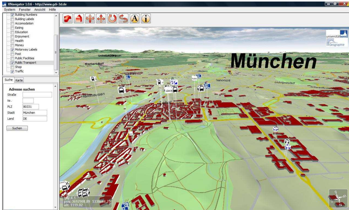
Figure 7: Web 3D Service for Germany based on open data (OSM) and SRTM DEM. Landuse, buildings and POIs generated from OpenStreetMap. The range of OpenLS services available from GDI-3D.de is available also in this application de offering OSM data in distinct ways from the integrated client XNavigator. Example: Munich.
