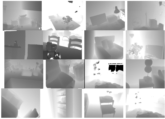
Fig. 1. Some representative rendered depth maps obtained from the 3D model generated using KinectFusion. These images give a general impression about the scenes in the dataset
