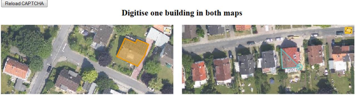
Figure 3. Prototype implementation of a Geo-reCAPTCHA client. Two map representations offer the possibility to digitise building boundaries in the form of polygons. The digitisation in the left map is already completed (yellow polygon) whereas the digitisation in the right map is currently in progress (blue sketch).
