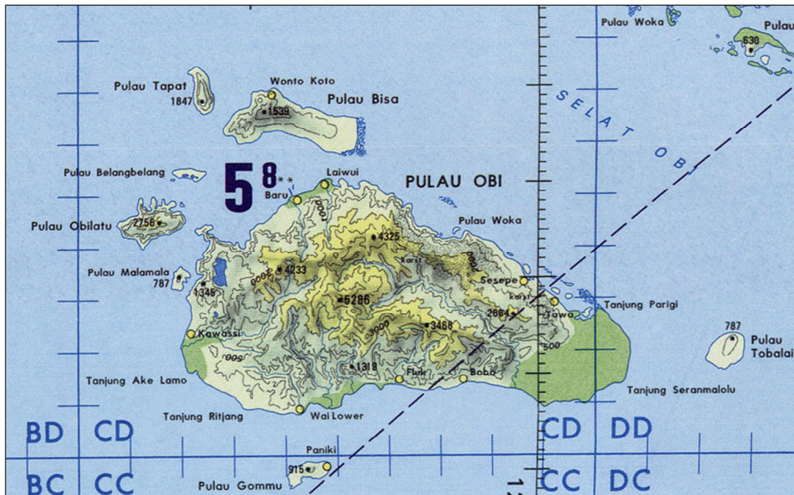
Figure 6.1. An example of manual lettering of Indonesian islands. Note how the multiple use of a full black and other dark print colours on the island’s interior (hill shading, height information, isolines, etc.) forces the ‘Pulau Obi’ and ‘Pulau Bisa’ labels to the outside of their polygons Source: Army Topographic Support Establishment (1997).
