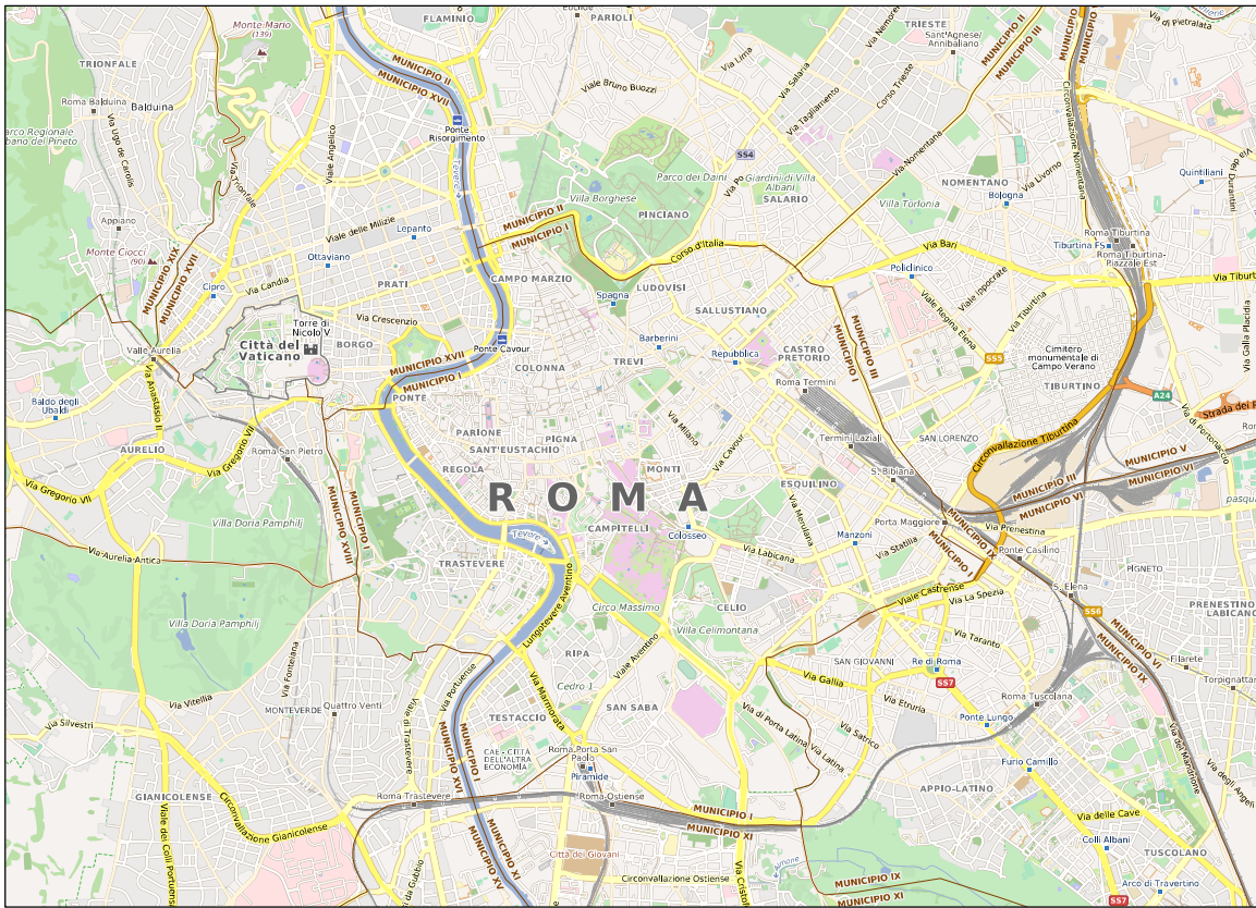
Figure 8.15. A sample map containing lettering of administrative boundaries together with other feature types such as roads, railways, districts, parks, etc. Projection: spherical Mercator (EPSG:3857). Data source: © OpenStreetMap contributors (2013, data licensed under ODbL).
