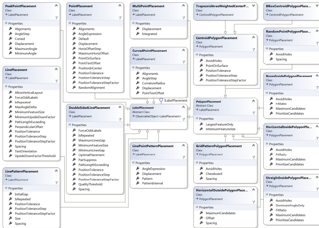
Figure 2.3. The diagram of label placement classes which are implemented in MapSurfer.NET. The classes PointPlacement , HorizontalOutsidePolygonPlacement , DoubleSidedLinePlacement correspond to the procedures for label-position generation in Chapters 5, 6, 8 respectively.
